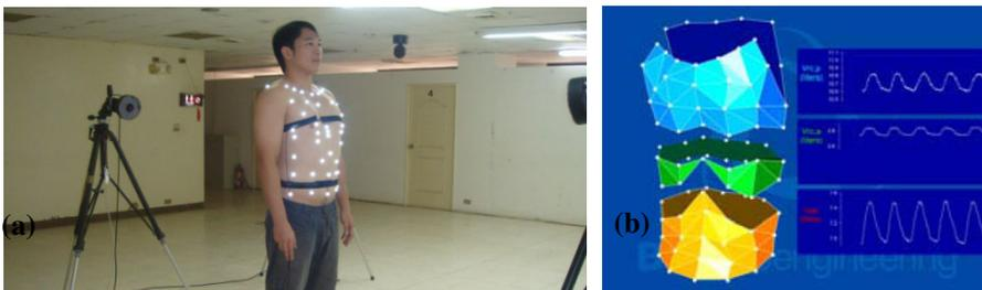
**Fig. 3.** Breath detection by using OEP equipment. (a) A participant is testing the breath pattern; (b) Detecting the breath pattern and visualized in real-time.
