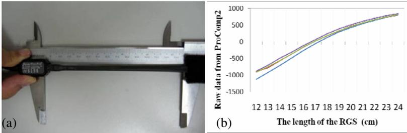
**Fig. 1.** Calibration of the RGS from raw data to the unit of length. (a) Using a ruler to calibrate the RGS every 0.5 cm; (b) The mapping table of the RGS four times.
